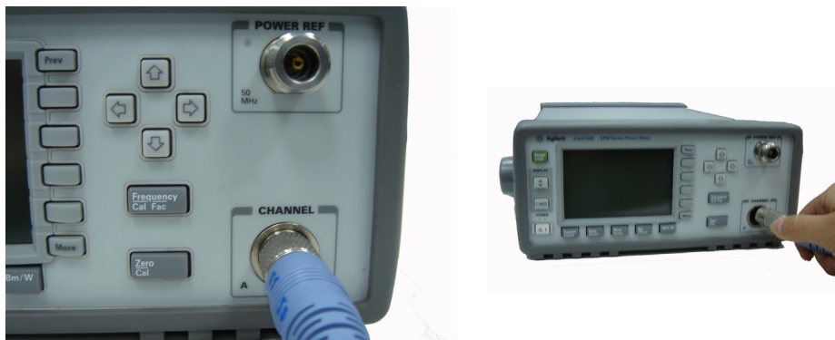
Figure 1-2 Connecting a sensor cable to power meter
